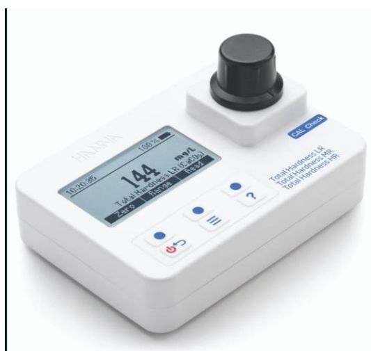
Fig 1. Aparatul Total Hardness Photometer MR [1]
