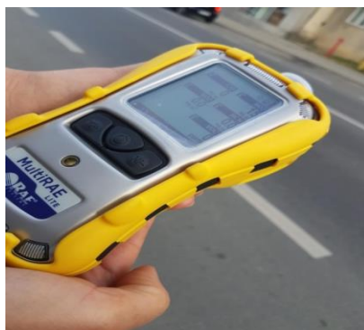
Fig.3. Monitorul MultiRAE wireless multi-gaz portabil
