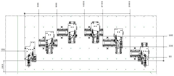
Fig. 7. Module fixing dimensions for a part
