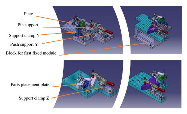
Fig. 5. The orientation and fixing subassemblies
