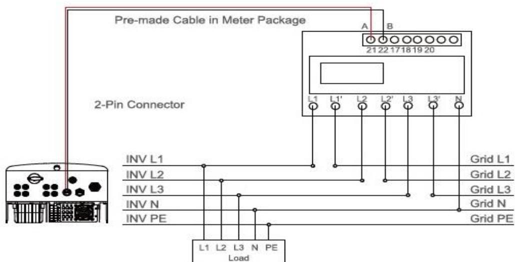
*Fig. 3. Connection diagram of a three-Phase with a smart meter*
