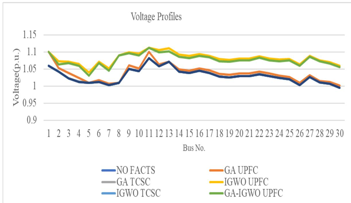
Figure 9: bus voltage profiles for different optimization techniques
