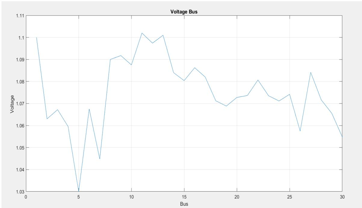
Figure 5: Voltage profile curve with IGWO-tuned UPFC
