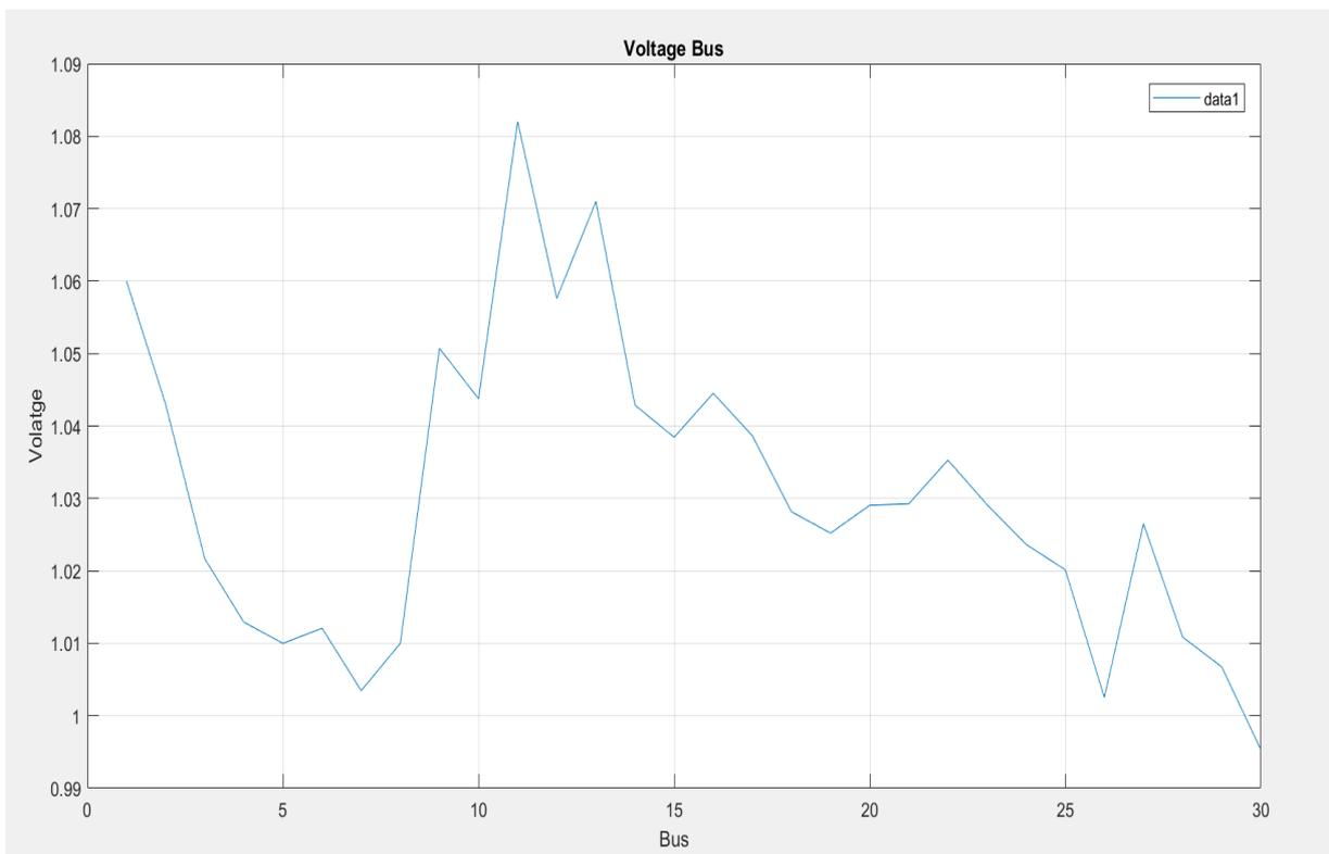
Figure 2: Voltage profile curve (Base case, without optimized FACTS)
