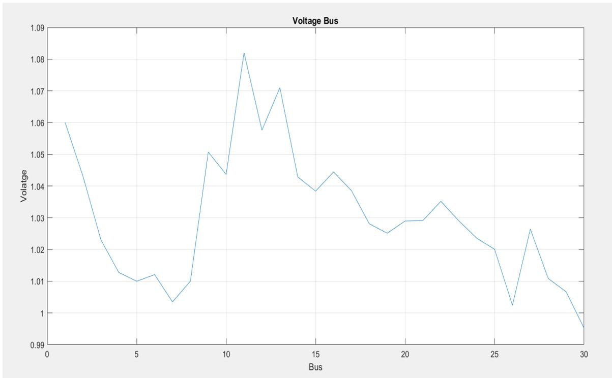
Figure 6: Voltage profile curve with IGWO-tuned TCSC
