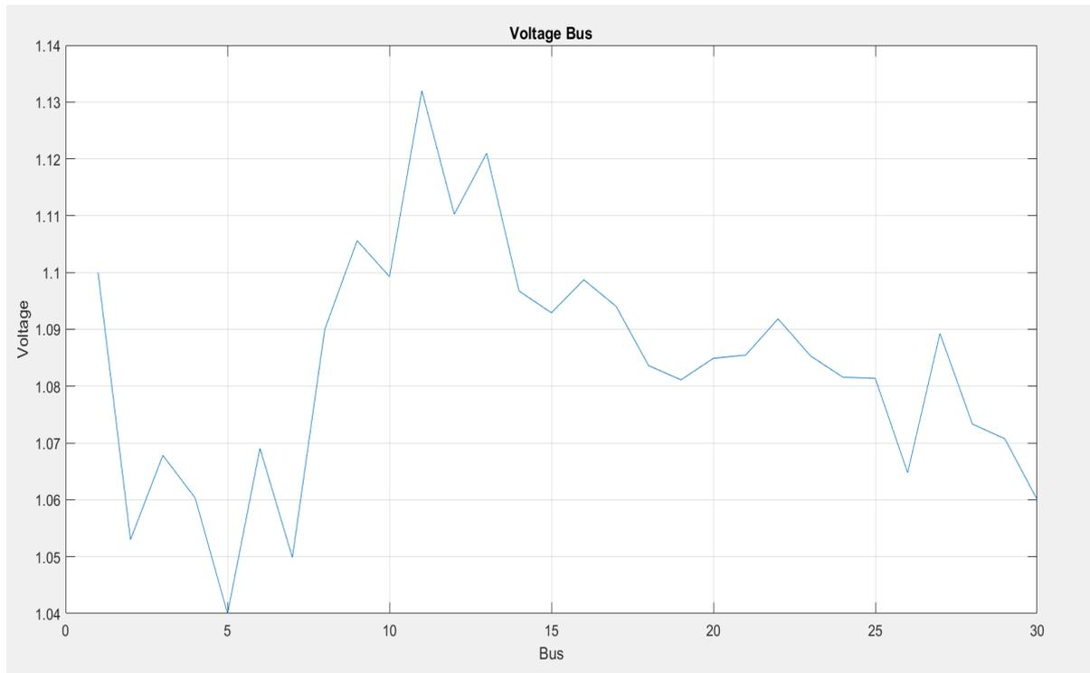
Figure 7: Voltage profile curve with Hybrid MGA and IGWO-tuned UPFC
