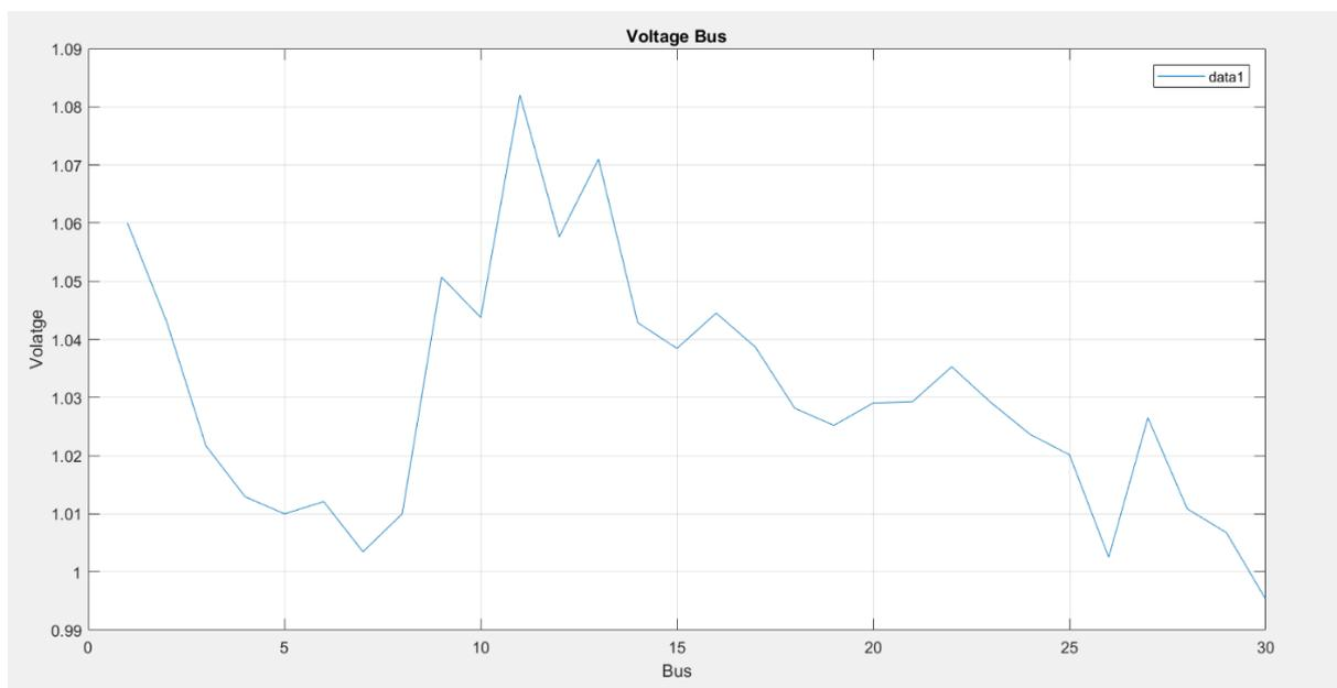
Figure 3: Voltage profile curve with GA-tuned UPFC
