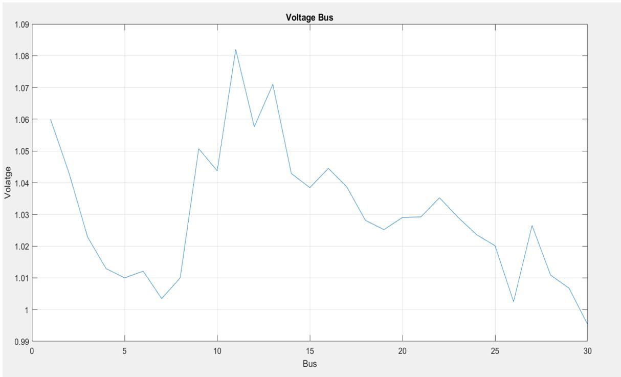
Figure 4: Voltage profile curve for the with GA-optimized TCSC FACTS Device
