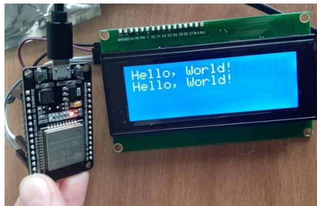
Fig. 17 Testing the display with ESP32 via I2C
