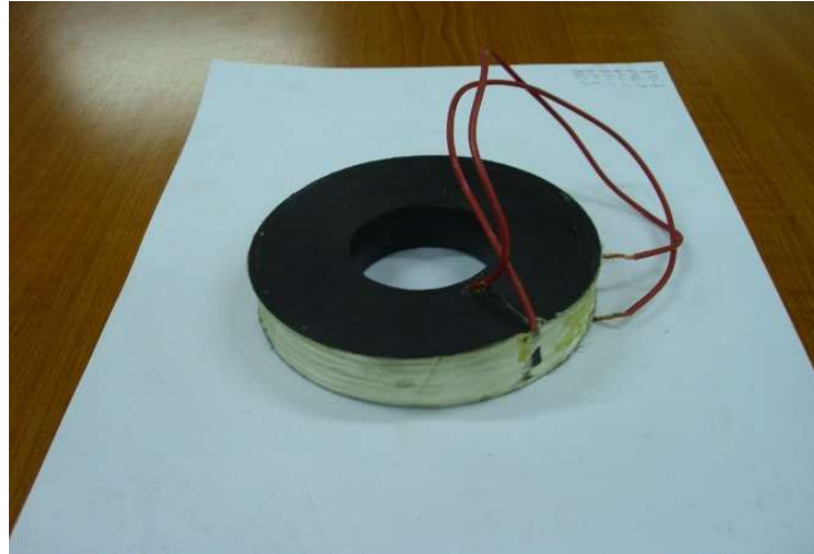
Fig. 2 The fixed coil of linear oscillating generator with moving permanent magnets
