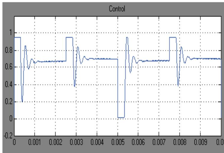
Fig. 7 The PI control signal of PWM generator.
