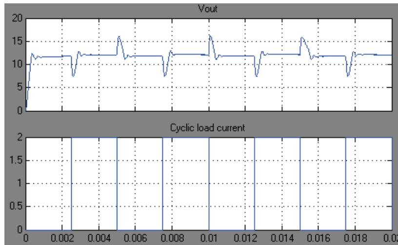
*Fig. 5 The stabilized  $V_{out}$  and the cyclic load current.*
