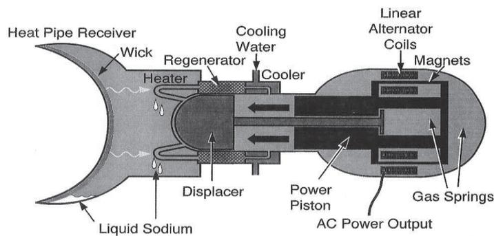
Fig. 2 Basic components of Beale “free-piston” Stirling engine [3].
