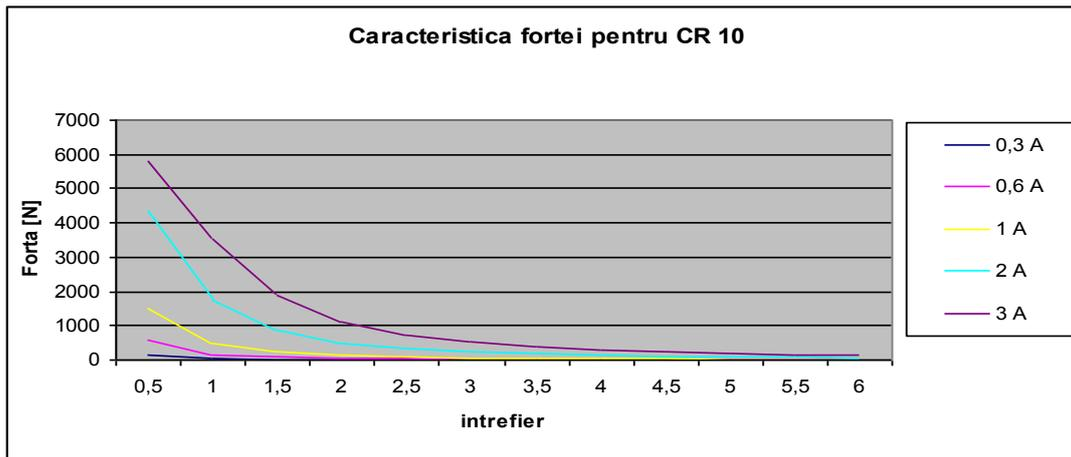
Fig. 5 Force characteristic for CR 10 and a current of 0.3 - 3 A
