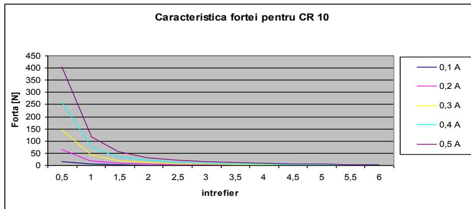
Fig. 4 Force characteristic for CR 10 and a current of 0.1 - 0.5 A
