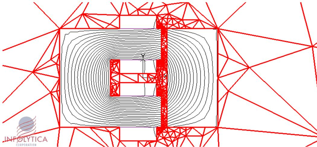
Fig. 2 The air gap mesh network
