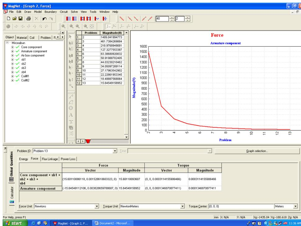
Fig. 3 Force characteristic for CR 10 and a current of 1 A
