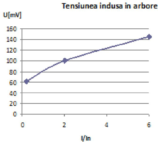
*Fig. 9.* The voltage induced by the starting current
