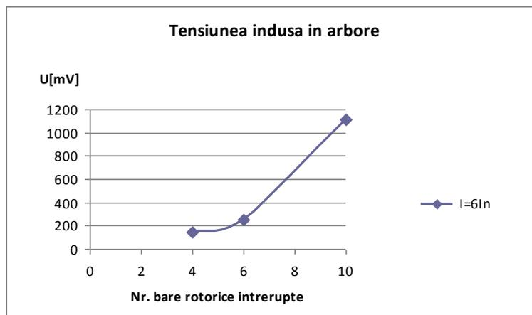
Fig. 5. Voltage induced on  $6I_n$
