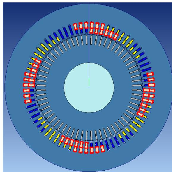
*Fig.2. Coils of phase*
