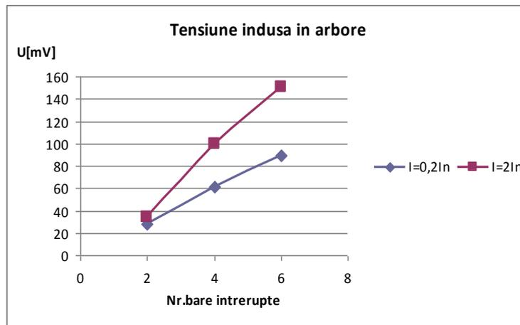
Fig. 4. The induced voltage according to the number of interrupted bars
