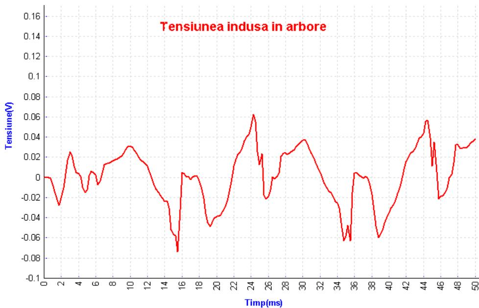
*Fig. 10.* The induced voltage form in the shaft
